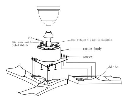
1) Lock the plate on motor, as shown in the figure below.
