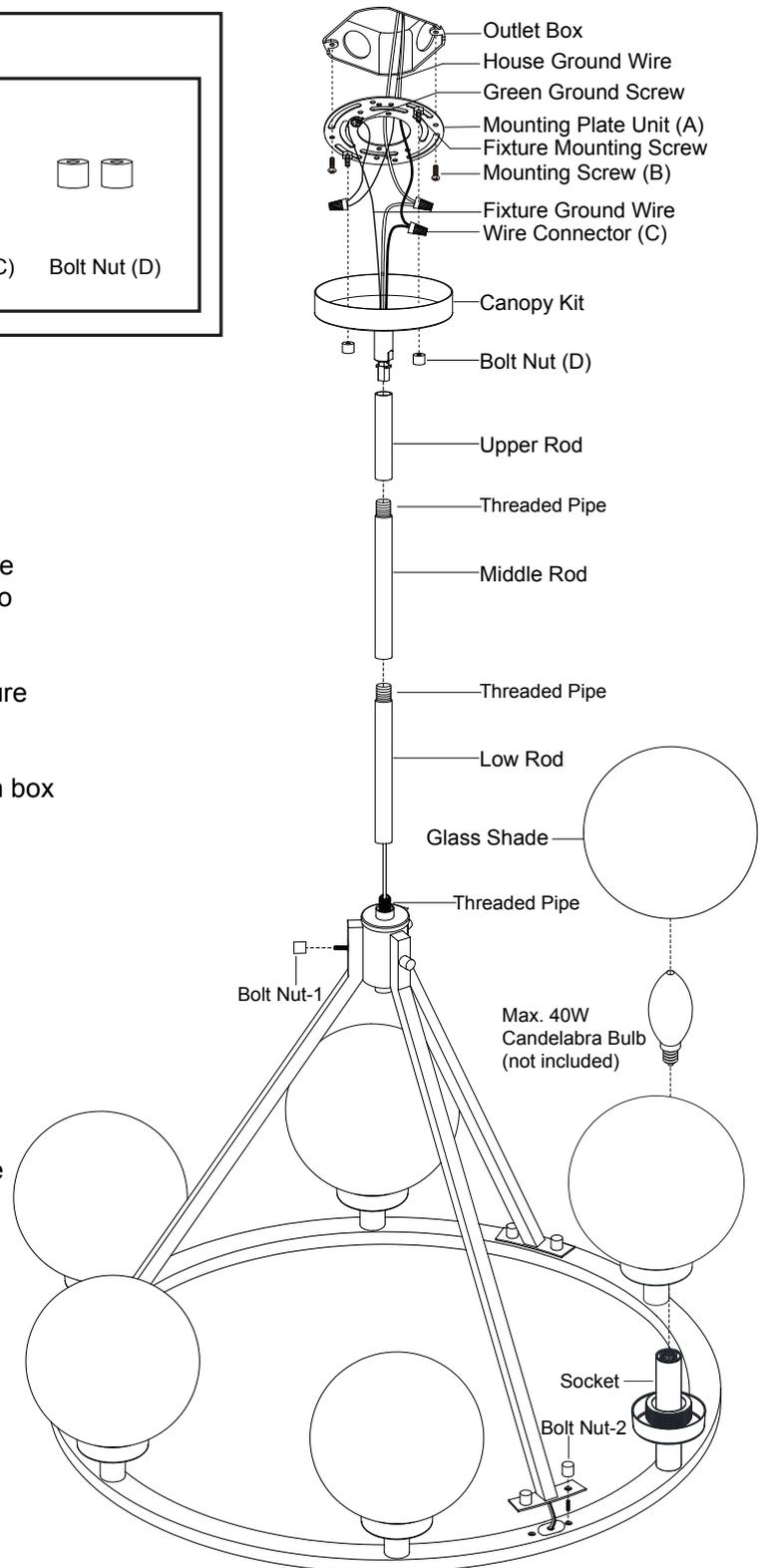
7. Pull out the source wires from the outlet box. Make wire connections using wire connectors (C) as follows:
