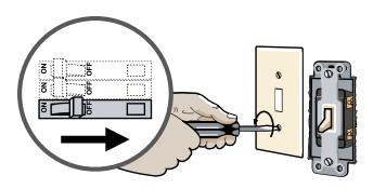
Step 1 Turn power OFF at breaker. Remove wallplate.
