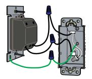
Step 3 Connect wires from box to dimmer.
