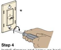
Install dimmer and screw on backplate.
