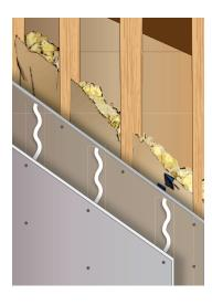
5 Apply gypsum wallboard staggering the joints so the edges do not fall onto studs and fasten to the 440 SB panel only (not through the studs) using #10 1-1/2" laminating screws (rock to rock screws).
