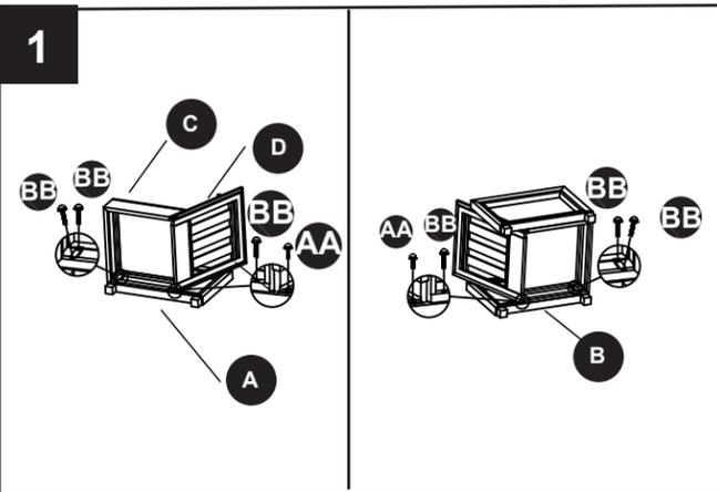
Once all connections are made, tighten AA, BB with CC.
