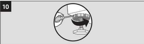
Once the washer is stabilized and does not vibrate, tighten the lock nuts on each leg of the pedestal using a flat head screwdriver.
