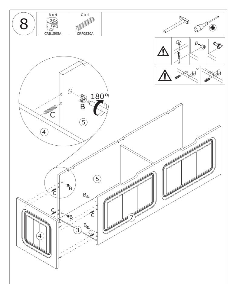
Attach board 4 to board 5 and 7 using wooden dowel(C), add cam lock(B) into board 5,7 and turn clockwise to tighten as shown.
