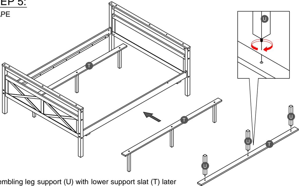
Assembling leg support (U) with lower support slat (T) later rotate, Move support slat inside Full bed.
