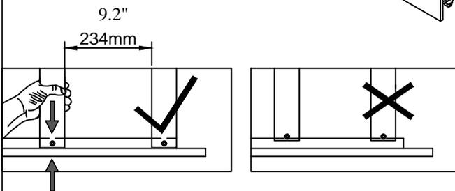
**NOTE:** Please make sure the bed slats close to the side rail before locking the screws to avoid breakage. This step is required for both the left and right sides. Moreover, please do not lock the screws of the bed slats at the outermost edge to avoid damaging.
