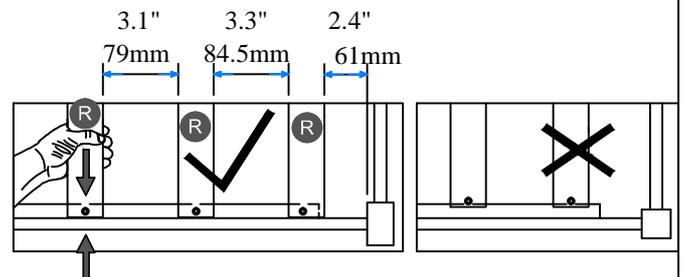
**NOTE:** Please make sure the bed slats close to the side rail before locking the screws to avoid breakage. This step is required for both the left and right sides. Moreover, please do not lock the screws of the bed slats at the outermost edge to avoid damaging.
