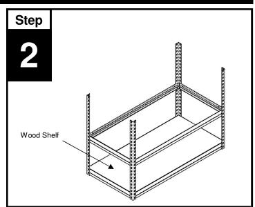
Start by adding a wood shelf to the level previously built, then continue working by adding the second level using two (2) beams and two (2) braces in the post slots of your desired location. Again place the rivets of the beams and braces into the post slots with the shelf ledge facing up and tap lightly to seat the rivets.
