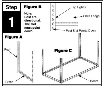
Assemble two (2) post with one (1) brace. Skipping one slot from the bottom of the post (see figure A), place the rivets into post with the slot pointing down, and with the shelf ledge of the brace facing up (see figure B). Tap lightly to seat rivets. Repeat with two (2) post and one (1) brace. Assemble the two (2) post units with two (2) beams (see figure C). Skip one hole from the bottom of post, tap lightly to seat rivets.
