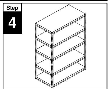
Add a wood shelf to the previously built level, then continue by adding the fourth and fifth level to the unit using two (2) beams and two (2) braces per level. Tap lightly to properly seat the rivets and add the final wood shelves to the unit.
