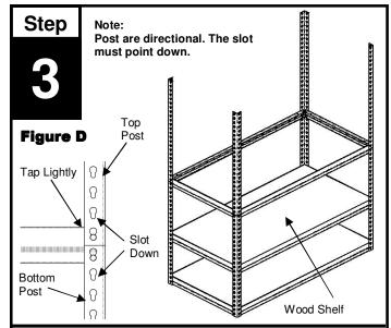
Add a wood shelf to the previously built level, then assemble the top post to the bottom post by using two (2) beams and two (2) braces. One (1) rivet from each beam and brace must be placed in the top hole of the bottom post, and the bottom hole of the top post (see figure D). After all beams and braces are in place, tap lightly to properly seat the rivets.
