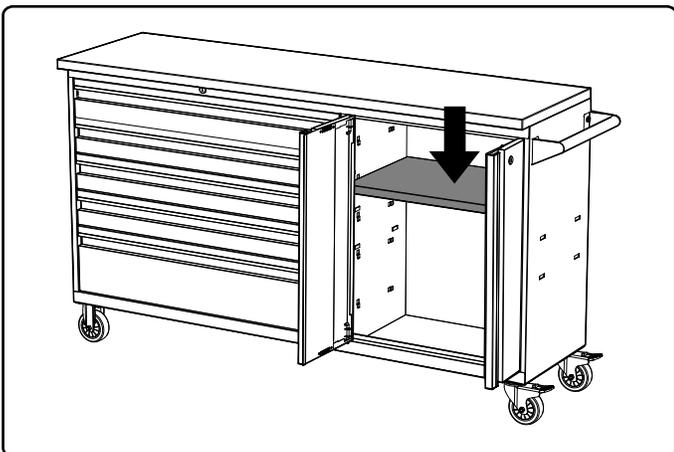
**4** Lower shelf onto brackets by sliding tabs into slots.
