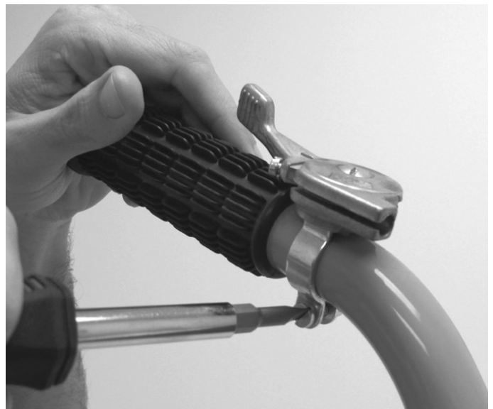
Step 4 – Attach the throttle lever to the handle, as shown above.
