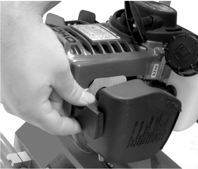
Step 1 – Remove carburetor cover by pressing clips.
