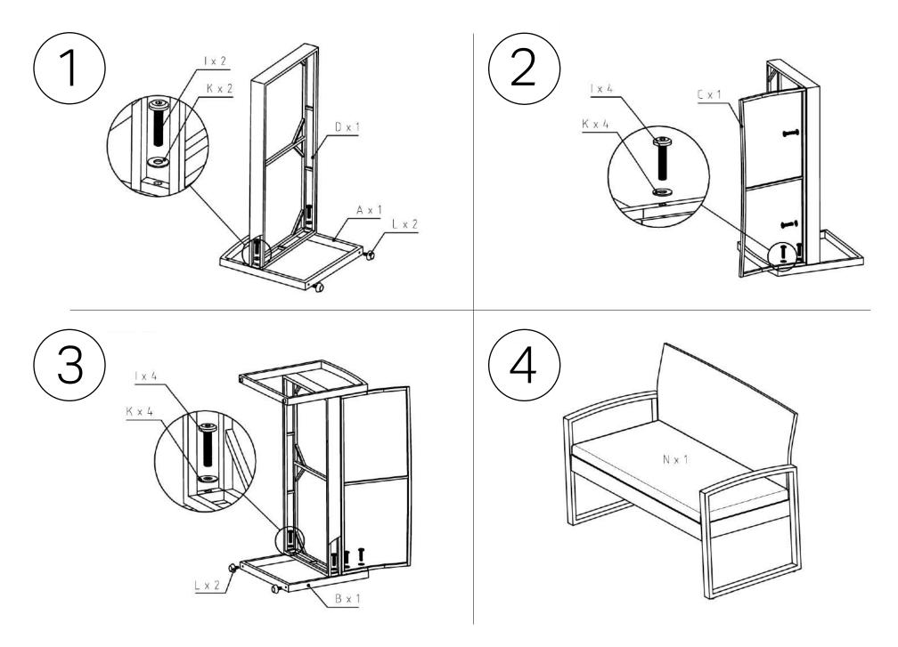
III- PRODUCT ASSEMBLY: CHAIR "DO NOT TIGHTEN THE SCREWS UNTIL ALL OF PARTS SET INTO CORRECT POSITION"
