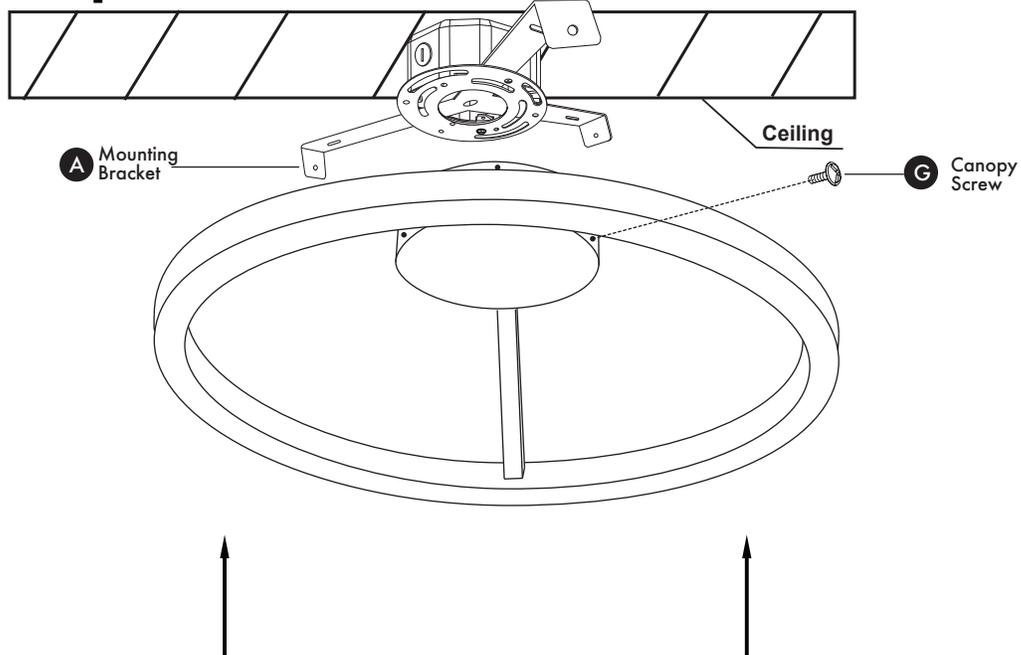
Attach fixture to mounting bracket (A).
