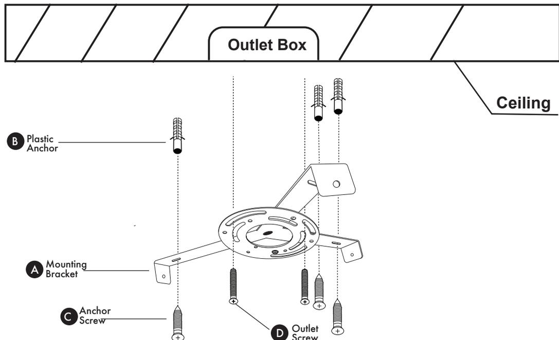
Attach mounting bracket (A) to outlet box with outlet screws (D). Screw anchor screws (C) into plastic anchors (B) to secure mounting bracket (A).
