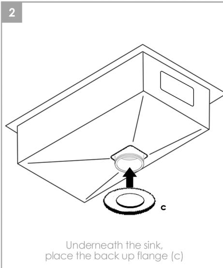
Underneath the sink, place the back up flange (c)
