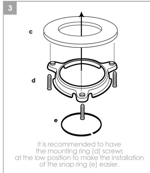
It is recommended to have the mounting ring (d) screws at the low position to make the installation of the snap ring (e) easier.
