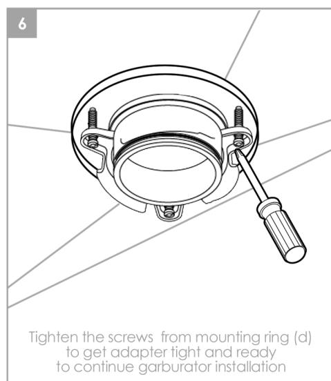
Tighten the screws from mounting ring (d) to get adapter tight and ready to continue garburator installation
