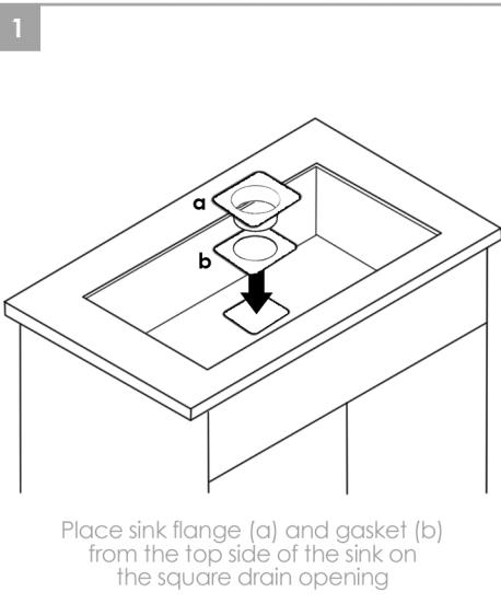
Place sink flange (a) and gasket (b) from the top side of the sink on the square drain opening
