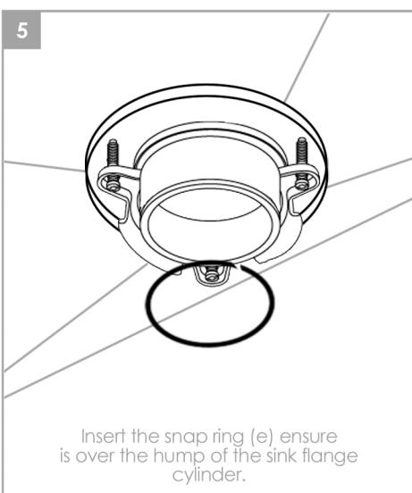
Insert the snap ring (e) ensure it is over the hump of the sink flange cylinder.
