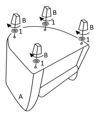
Place Chair (A) on its back on a flat smooth surface. Attach Feet (B) and Washers (1) to Chair (A).
