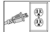
Double insulation eliminates the need for a three-wire grounded power cord and grounded power supply system. This is applicable only to Class II (double-insulated) tools. This power tool is a double-insulated tool.
