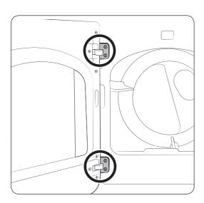
11. Reinstall the door on the front frame, and then carefully insert and tighten the 4 hinge screws.
