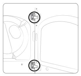
To reverse the direction of the door, we recommend that you contact a qualified technician. It is recommended to put a soft rug on the floor to prevent scratches on the door.
