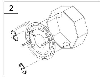
2. Attach this assembly to the outlet box using the mounting screws supplied with the outlet box (not provided). Tighten securely.
