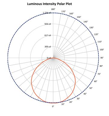
ral ---- Horizontal Cone Through 2.5-Deg Vertical
