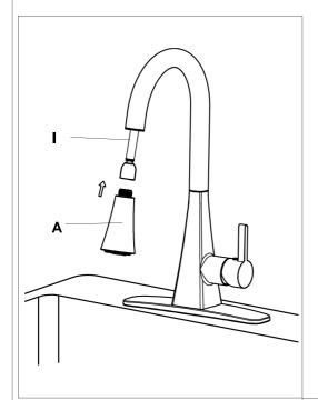
Step 9: Pull out the pull hose (I) the faucet outlet, and then tighten the sprayer (A) on the pull hose (I).
