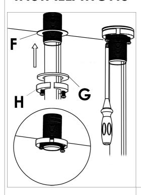
Step 2: Firstly, thread the rubber gasket (F), silver gasket (G) and metal gasket (H) from the pull hose under the sink in order, and then tighten the two screws with a cross screwdriver to fix the upper part of the faucet.
