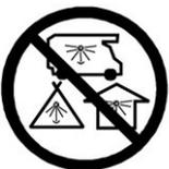
This appliance can produce carbon monoxide which has no odor. Using it in an enclosed space can kill you. Never use this appliance in an enclosed space such as a camper, tent, car or home.
