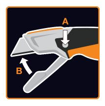
If the blade is exposed, press the button on the side of the knife (A) to engage the blade guard (B).
