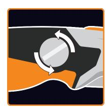
2. Turn the circular lock counter-clockwise until the handle springs open.
