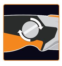
Close handle and turn the circular lock clockwise until it's tightened.
