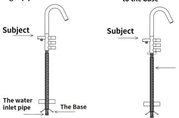
3. Screw and hand tighten the water inlet pipe to the water inlets of the subject (DO NOT USE SPANNER TO TIGHTEN AS IT CAN DAMAGF THE O-RING) Make sure the water inlet pipe were screwed into the correct inlets for hot water and cold water.
