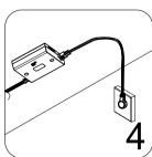
Make sure the on/off button is in the off position. Plug the power cord into an electrical outlet and insert the other terminal into INPUT port of the switch.
