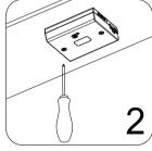
Pay attention to INPUT and OUTPUT direction. The Power Cord will connect to the INPUT side. Hold in place and insert mounting screws. Provided screws are suitable for cabinet bottoms 3/8in. or thicker. Pre-drill a pilot hole for the screws using a 3mm or 1/8in. size drill bit if needed.
