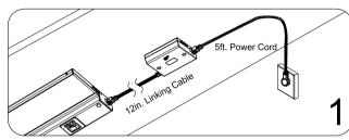
Place the product in the desired position. Ensure the 5ft. Power Cord (included with your bar or puck) can reach the outlet and that the 12in. Linking Cable (included with this package) can reach the nearest bar or puck. If your layout exceeds the distance between each fixture, swap the 12in. linking cable for longer versions (sold separately).
