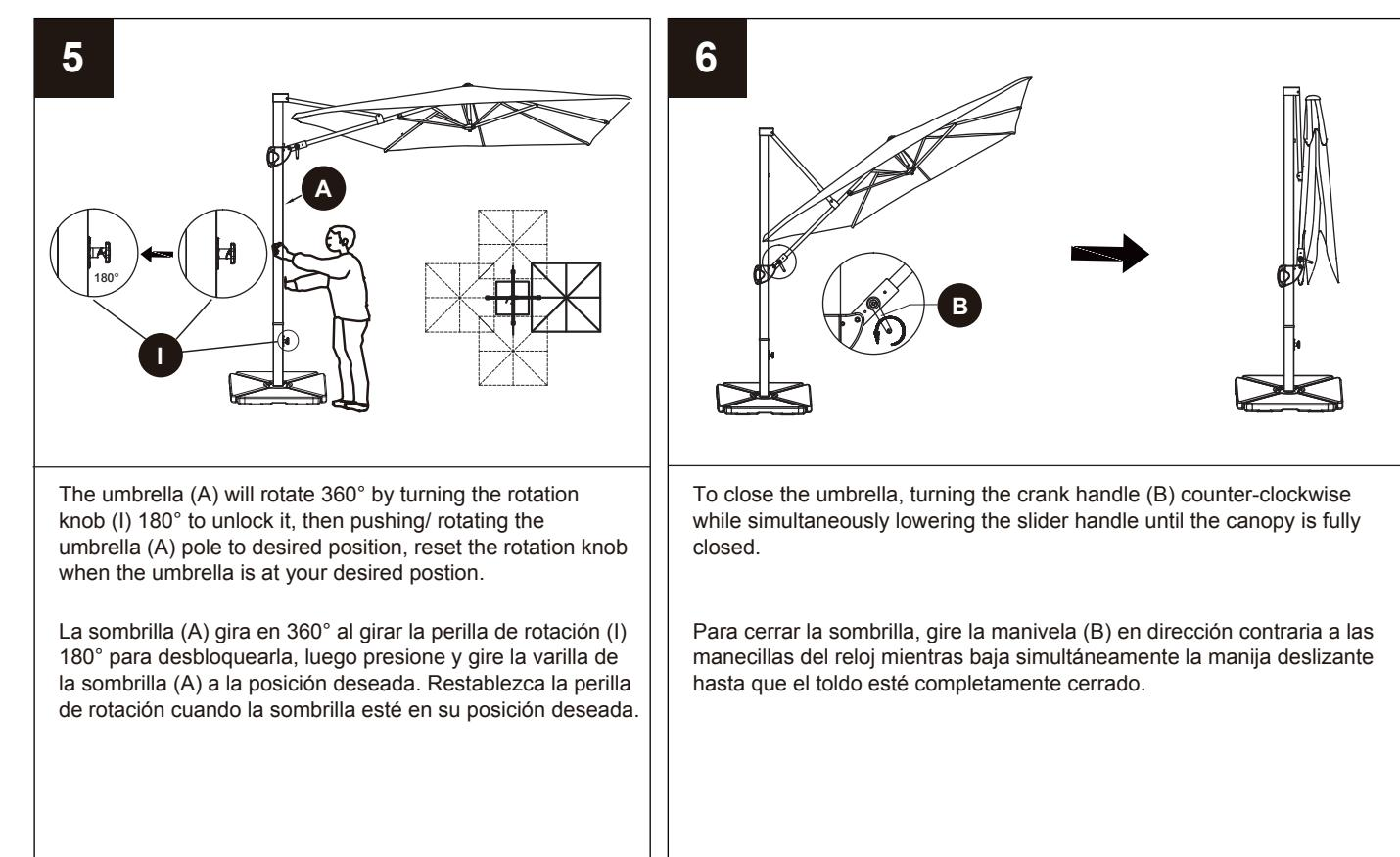
The umbrella (A) will rotate 360° by turning the rotation knob (I) 180° to unlock it, then pushing/rotating the umbrella (A) pole to desired position, reset the rotation knob when the umbrella is at your desired position.
