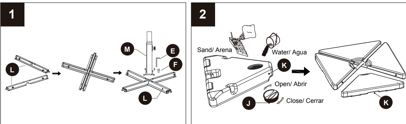
Assemble the metal stand (L) by overlapping the metal bars together on the ground in a cross pattern as shown. Then Line up the mounting holes in the bottom pole (M) on top of the metal stand (L). Secure the bottom pole (M) to the metal stand (L) with 4 pcs bolt for base (F). Tighten with the large wrench (E).
