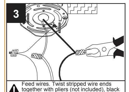
**! Feed wires. Twist stripped wire ends together with pliers (not included), black to black, white to white, and ground/bare to ground/bare.**
