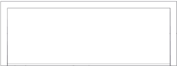
D10 WINDOW FRAME - W4L20629 (x2) 1 7/16"x4 3/16"x11 7/16" (36x106x290)
