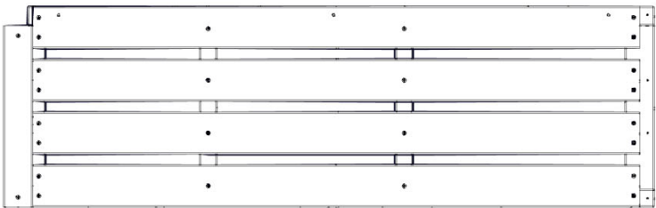
TB01 TABLE ASSEMBLY - W2A04439 (x1) 2 1/16"x16 1/16"x51 15/16" (52x408x1319)
