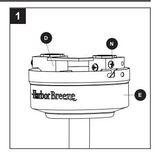
Secure the canopy (E) with the mounting bracket screws (N) previously removed (Step 4, page 8).
