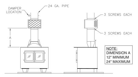
12. Again, do not install your Miracle Heat closer than 18" from any combustible material.
