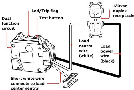
**NOTE:** The neutral pigtail on eMBC's (AFCI, GFCI and DFCI) can be cut to length in the field or extended using approved connectors. Additionally, eMBC's with shortened neutrals can be installed as shown providing a fast and clean installation.
