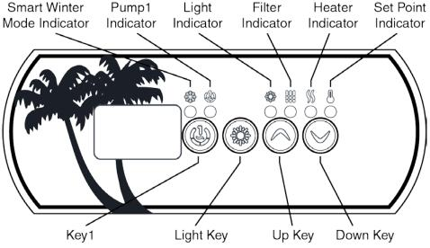
**NOTE:** Same control is used for 1 speed pump and 2 speed pump spas.
