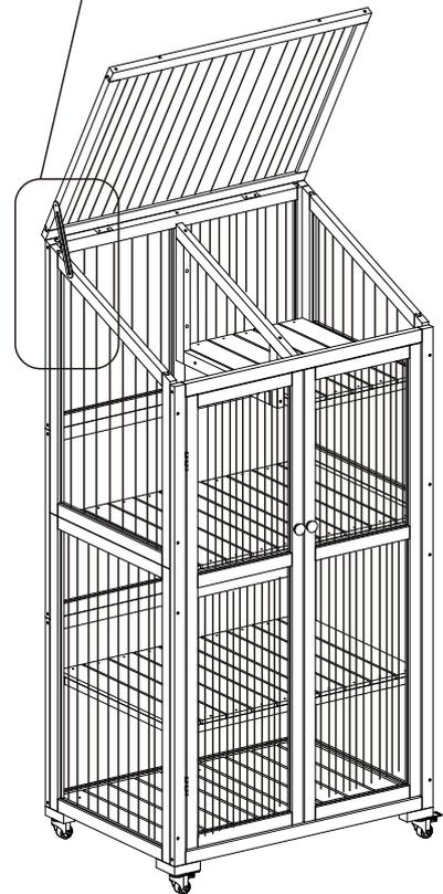
Remove 4 wheels firstly ,then assembly L shape metal and nails.
