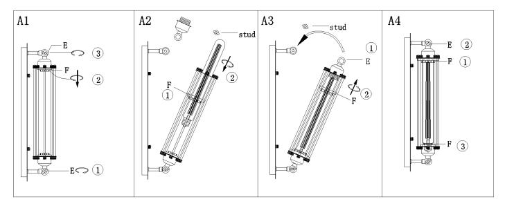
Step A1: Unscrew the lower stud to loosen the hinges making it feel like it's going to fall apart Remove the upper ring (F)from socket, then unscrew the stud from joint (E)
