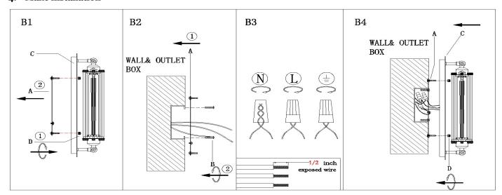
Step B1:Unscrew ball nuts (D)from the back plate(C) then remove the moungting plate(A)
