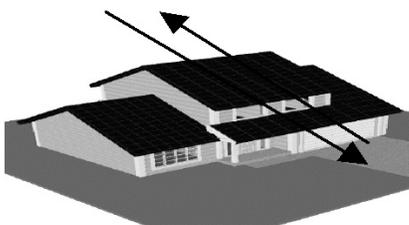
**Step 3.** Measure 9 inches from a wall that is parallel to the direction of the joist. This is a good starting point that should be very close to the joist. Or if you have a heat vent in the floor you can use that to find the joist. The vent is always between two joists. If you were to start next to the vent you will probably find the joist on the first or second attempt. Drive the Joist Finding Screw down into the floor 2 inches.
