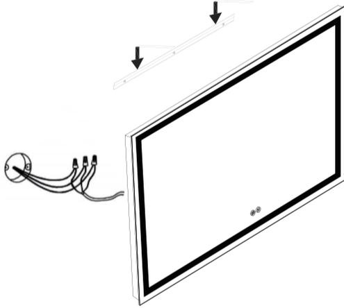
**Warning:** Strip wires to a suitable length. DO NOT connect the hardwire to a plug & socket outlet
