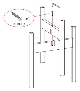
Assemble the plant holder by using Screw (RF10003) as shown.
