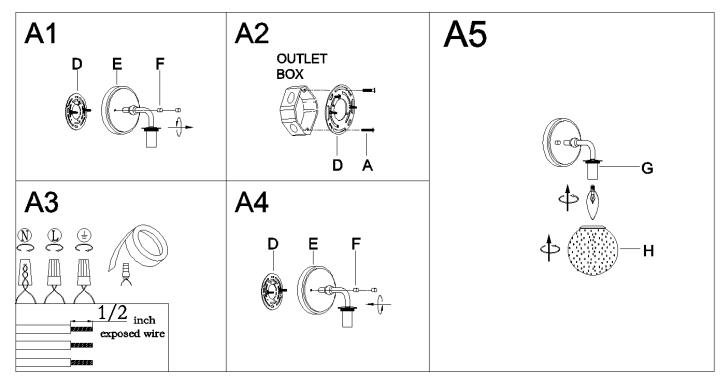
Step A1: Unscrew knob nuts (F) from mounting plate (D), then set aside for the following steps.
