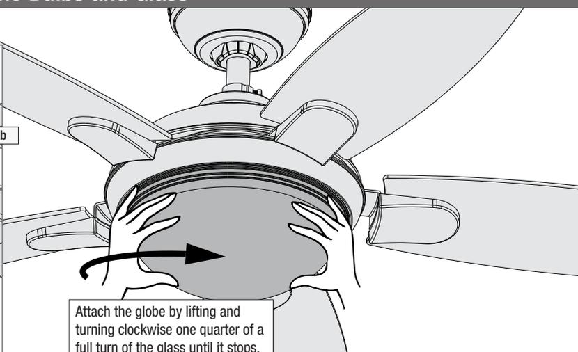
Attach the globe by lifting and turning clockwise one quarter of a full turn of the glass until it stops.
