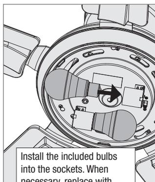
Install the included bulbs into the sockets. When necessary, replace with bulbs of same wattage.
