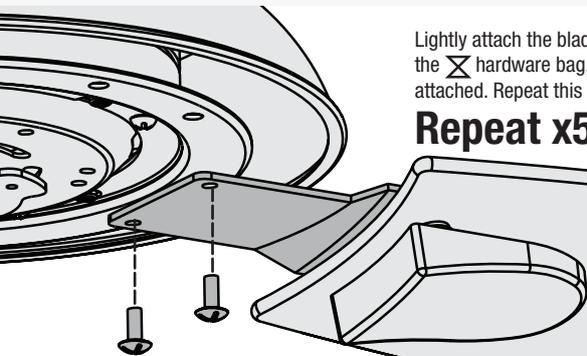
Lightly attach the blade irons to the motor with screws found in the ✕ hardware bag, then securely tighten after both screws are attached. Repeat this step for each blade assembly.
