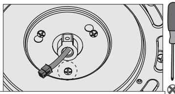
After rotating the light fixture into place, tighten all three screws securely.
