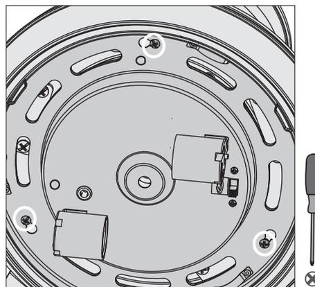
After rotating the light fixture into place, tighten all three screws securely.
