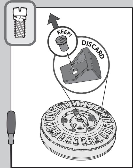
⊗ Remove the shipping blocks from the motor. **Save the screws. They will be needed for blade iron installation.**
