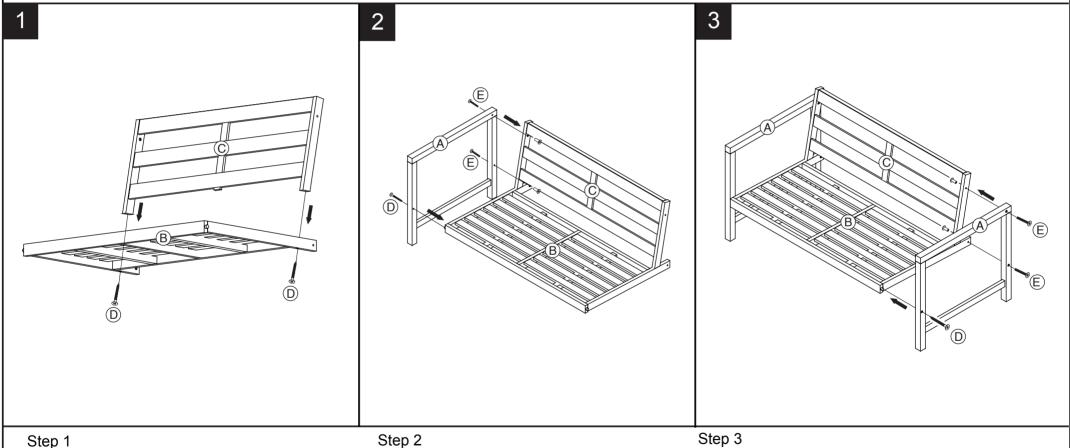
Attached seat frame (B) to (C). Using Screw (E) tighten by (F).
