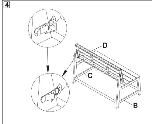
Step 3: attach the back (D) to the side as shown on the picture use the Allen bolt (F2). Tighten by the Allen Key (F3) and wrench (F4) as shown on the picture. Make sure to put correct position hardware each position. This step show this bench can use the back (D) same table.
