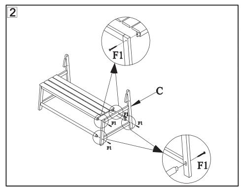
Step 1: attach the right side (B) to the seat (A) and the joint bar (E) as shown on the picture. Then use the Allen screw (F1) to tighten all points by using the Allen Key (F3).
