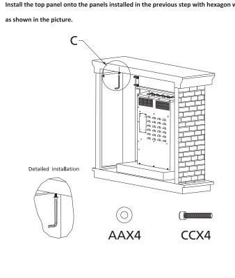
Note: Tighten all the screws completely after assembly.
