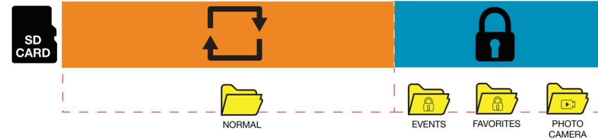
Once the SD card is full, the dash cam will continuously overwrite the oldest footage recorded with recent recordings. To protect a clip so that it will not be overwritten, press the Action Button so that the clip is moved into the locked content partition.
