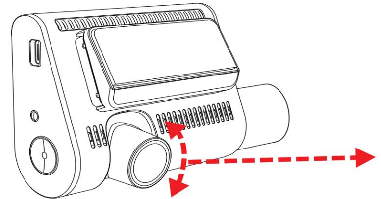
Rotate front dash cam lens so that it is parallel with the road.
