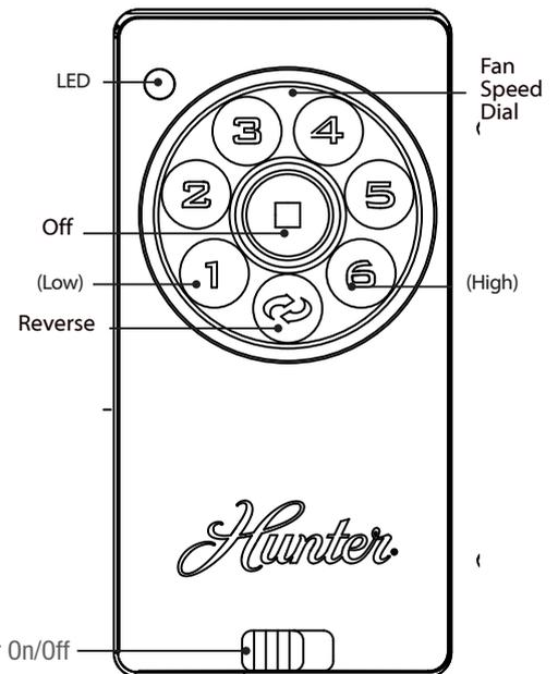
To select fan speed press one of the numbers on the Fan Speed Dial. To calibrate the fan speed, run the fan on "6" for 90 seconds after each AC power reset. The LED light flashes to indicate a signal has been sent to the fan. To reverse the air flow direction, press the Reverse button while fan is running.
