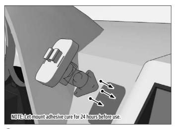
2 Attach the holder to the mount by inserting the Dual T-Tabs of the mount into the holder.
