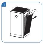
① Clasp the grooves of the left and right side panels by hand and pull diagonally upward and outward.
