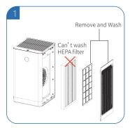
① Remove the air intake grilles and pre-filters.
