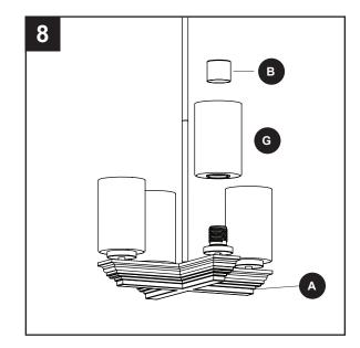
Install the E26-base bulbs (sold separately) into the socket of the fixture. **Note:** Fixture is compatible with any E26-base LED, CFL, or incandescent bulb (60 watt max.).
