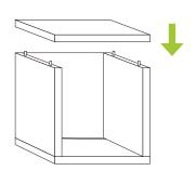
Align horizontal zBoard and press firmly to secure unit together.
