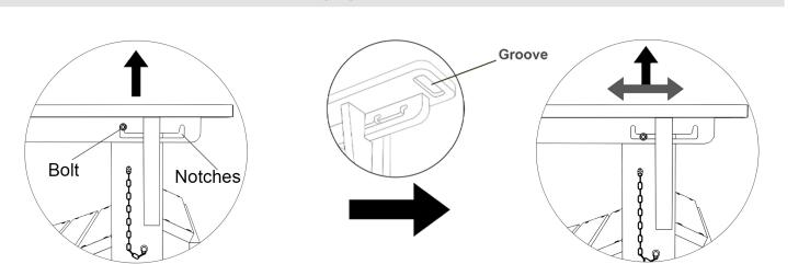
You must lift the armrests and pull them backward or forward to adjust the backrest angle. There is a small groove at the bottom of the armrest where your fingers should go when you lift the armrests.
