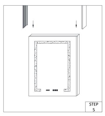
The side panels and cabinets are individually packaged, you need follow the STEP 5 to STEP 7 to install the side panels for hanging walls version, for embedded installation no need install the side boards.
